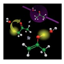
Baby steps: The mechanism of proton migration in an ionized acetone—water cluster was studied by IR spectroscopy. After the ionization, water abstracts a proton from the methyl group of the acetone moiety and transfers it to the carbonyl group (see picture).
