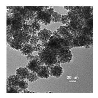
Flower power: A universal approach is presented for high-yield synthesis of Au, Pt, and Pd nanoflowers using the surfactant sodium *N*-(4-*n*-dodecyloxybenzoyl)-Lisoleucinate (SDBIL). The pH-dependent self-assembly using SDBIL is critical for nanoflower growth. The Pt and Pd nanoflowers show superior catalytic activity for Suzuki–Miyaura and Heck coupling reactions over spherical counterparts.
