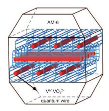
Vanadosilicate zeolite AM-6, which contains a 3D array of vanadate (VIVO32-) quantum wires (see picture), was prepared as high-quality crystals (free from V<sup>V</sup>, titanosilicate seeds, and pore-blocking organic template cations) from inexpensive  $V_2O_5$ . The linear dependence of  $\lambda_{max}$ and band-gap energy  $E_g$  on the partial charge on the framework O atoms reveal that the UV band of AM-6 is due to VIV-to-O metal-to-ligand charge transfer.
